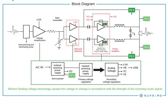
The Adaptive Voltage Switching Power Supply is the most innovative SMPS design introduced by NuPrime. The amplifier's output signal feeds back into the power supply's servo power stage, causing a change in the output voltages supplying the power stage of the amplifier. This design resulted in more details at a low music level and explosive power at a high volume.
